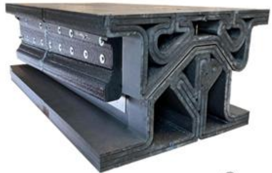
Figure 6.0. Complete AM ABS/Sheet metal Clad, Compression Mold Set.
