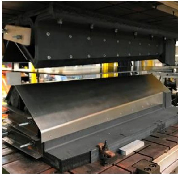
Figure 6.0 AM mold set in press. Sheet Metal cladding is clearly visible on the plug mold.
