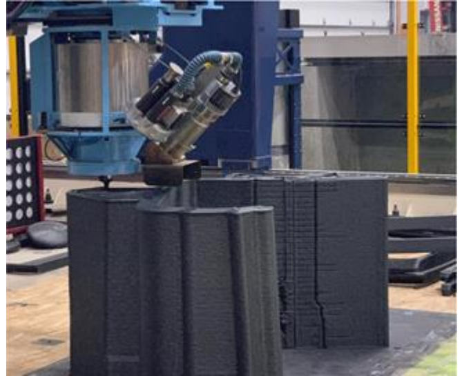
Figure 5.0 Two Large Scale AM molds being printed in one file then separated
